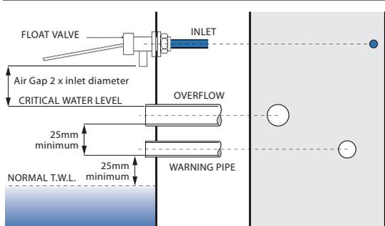
**Fig. 11a:** Relative positions of inlet, warning pipe and overflow for type 'AG' and 'AF' air gaps.
