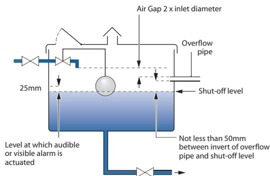
Fig. 11d: Cistern capacity greater than 5000 L – Type AG' and AF'
